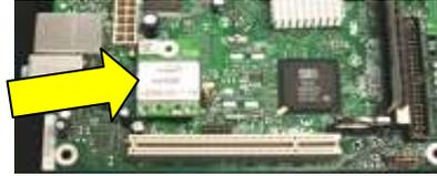
3.) Flash drive on motherboard Option. It is a small push-on board with a decal. If the version is less than 1.21, this flash drive will have to be replaced. Unplug game and remove Flash drive from motherboard. Install new flash drive by covering all pins and pushing straight down.
